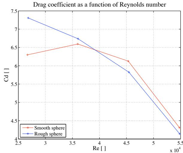
Figure 8: Drag force on smooth and rough sphere as a function of Reynolds number
