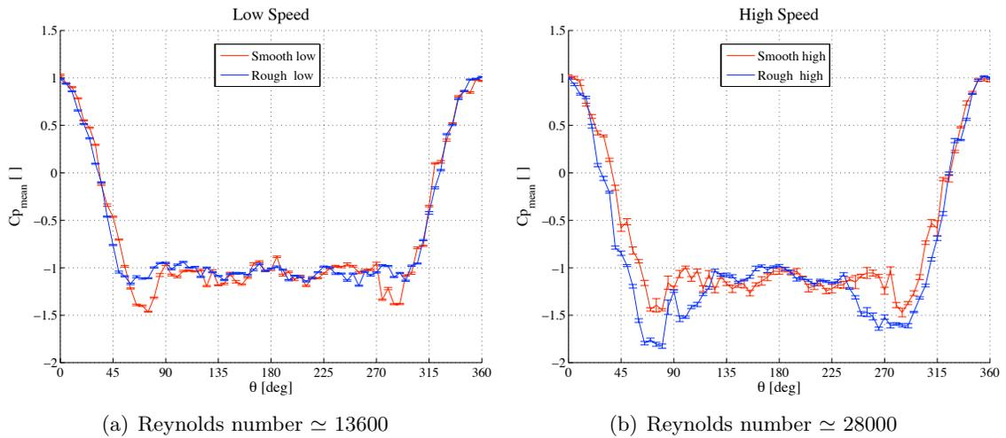
Figure 6: Pressure coefficient around the smooth and rough sphere with uncertainty intervals
