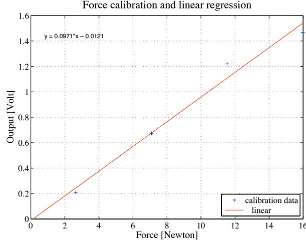
Figure 5: Linear regression on force calibration data
