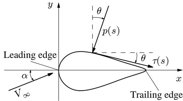
Figure 1: Nomenclature for pressure and shear stress distribution
