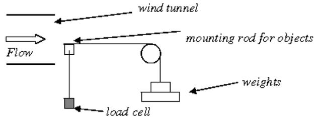
Figure 3: Setup for calibration of force balance
