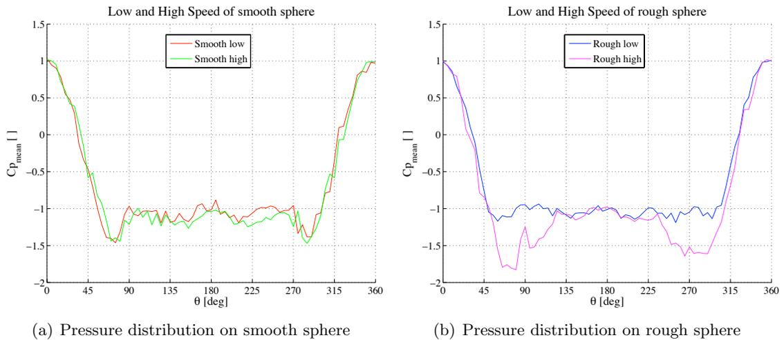
Figure 7: Pressure distribution as a function of Reynolds number for smooth and rough sphere
