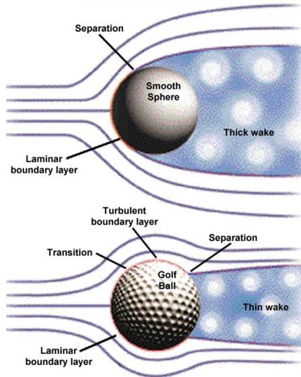
Figure 2: Viscous flow over a smooth Sphere and a Golf Ball, [1]
