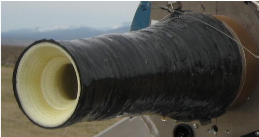
Figure 7- CCA showing Silica Fiber Ablative & Carbon overwrap
