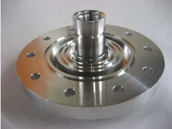
Figure 5- Machined injector bottom plate showing o-ring grooves (left) & orifices on the face of plate (right)
