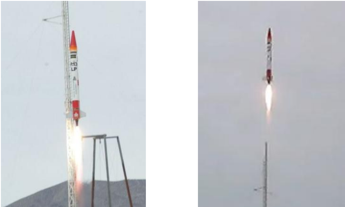
Figure 11: P-13 LP climbing the launch rail (left) & first ever flight using LOX/propylene (right)
