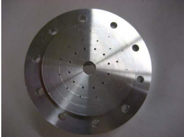
Figure 5- Machined injector bottom plate showing o-ring grooves (left) & orifices on the face of plate (right)
