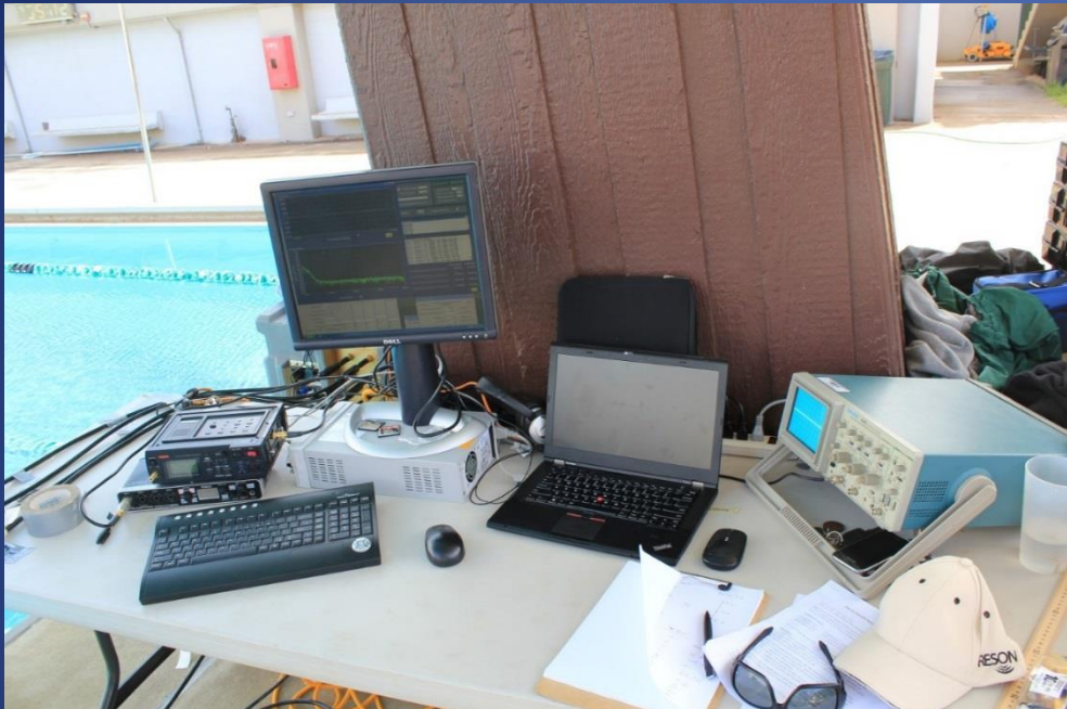
Fig.4: Reverberation experiment: Playback and recording equipment
