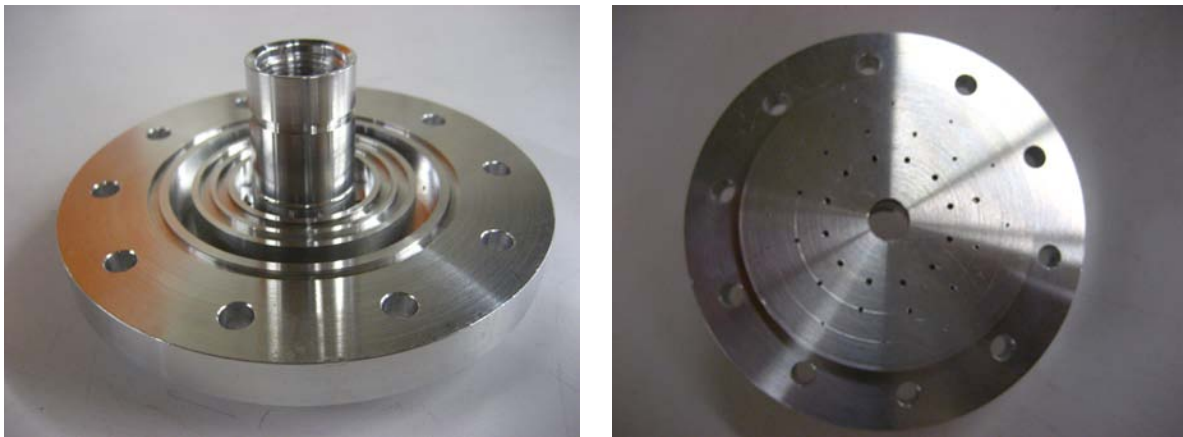
(a) Bottom Plate, showing O-ring Grooves
